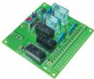
Line control gear motor control card
