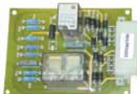
Gear motor control card
